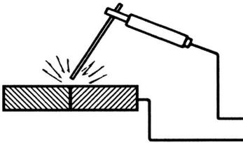
*Figure 1.1 Principle of Manual Metal Arc (MMA) welding.*
