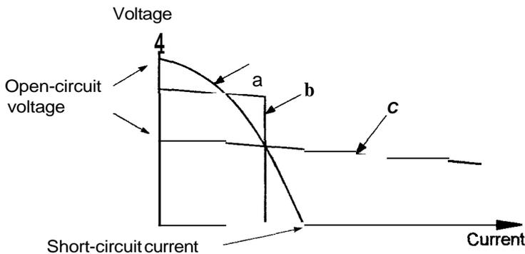
Figure 1.20 Examples of a) a drooping characteristic, b) a constant-current characteristic and c) a straight or slightly drooping characteristic.
