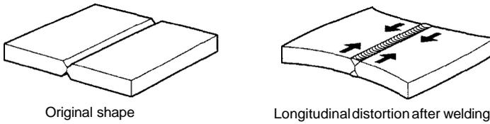
Figure 1.12 Longitudinal distortion.
