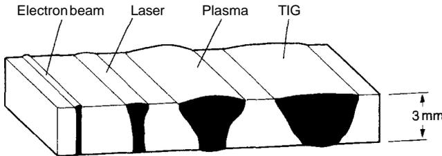
Figure 1.14 Penetration profile for some different welding methods.
