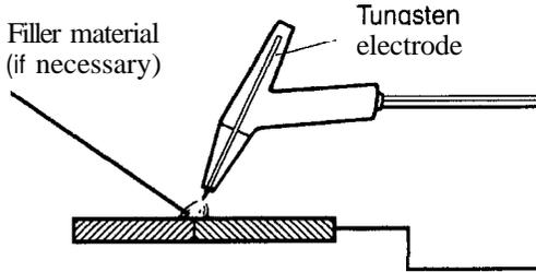
*Figure 1.3 The TIG welding method.*
